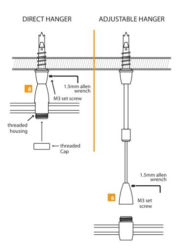
11 Tighten the M3 set screw on the conical nipples with the 1.5mm Allen wrench.
